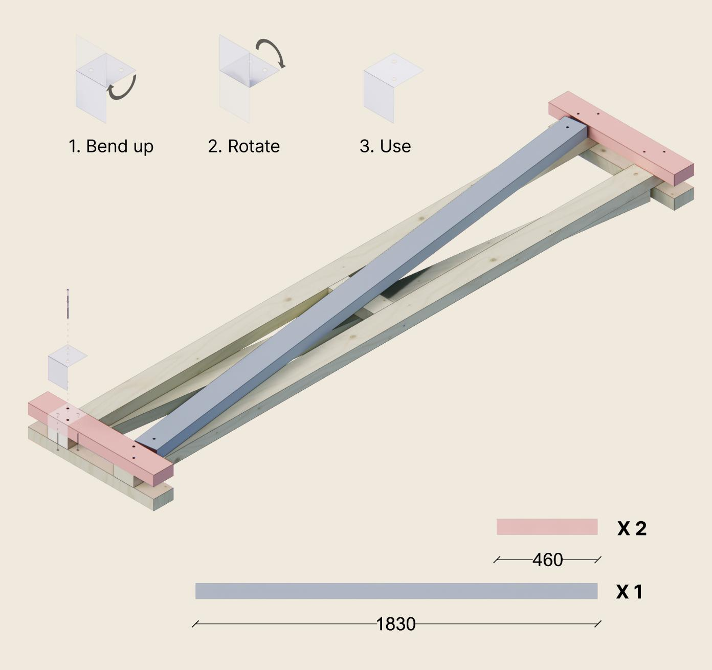
To avoid collision with the screws from the previous step, flip the diagonal template as shown below, and mount the screws as indicated.
