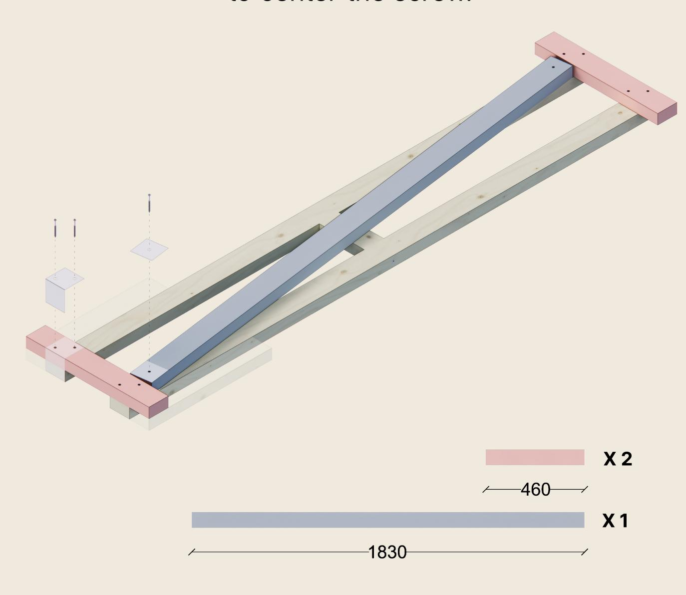
Use other battens at both ends to place the pink batten. Ensure that the end of the pink batten is flush with the other battens, as illustrated.
