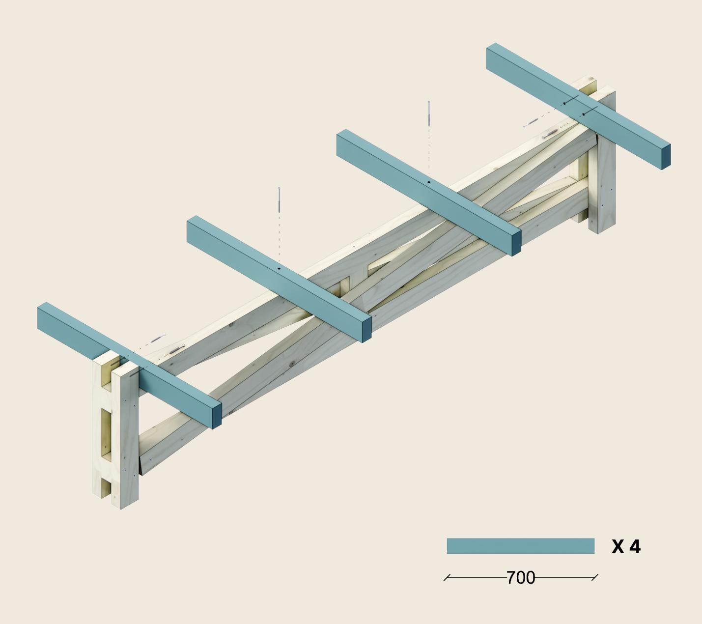
Use long screws for the two middle ones and short screws for the ones in each end.
