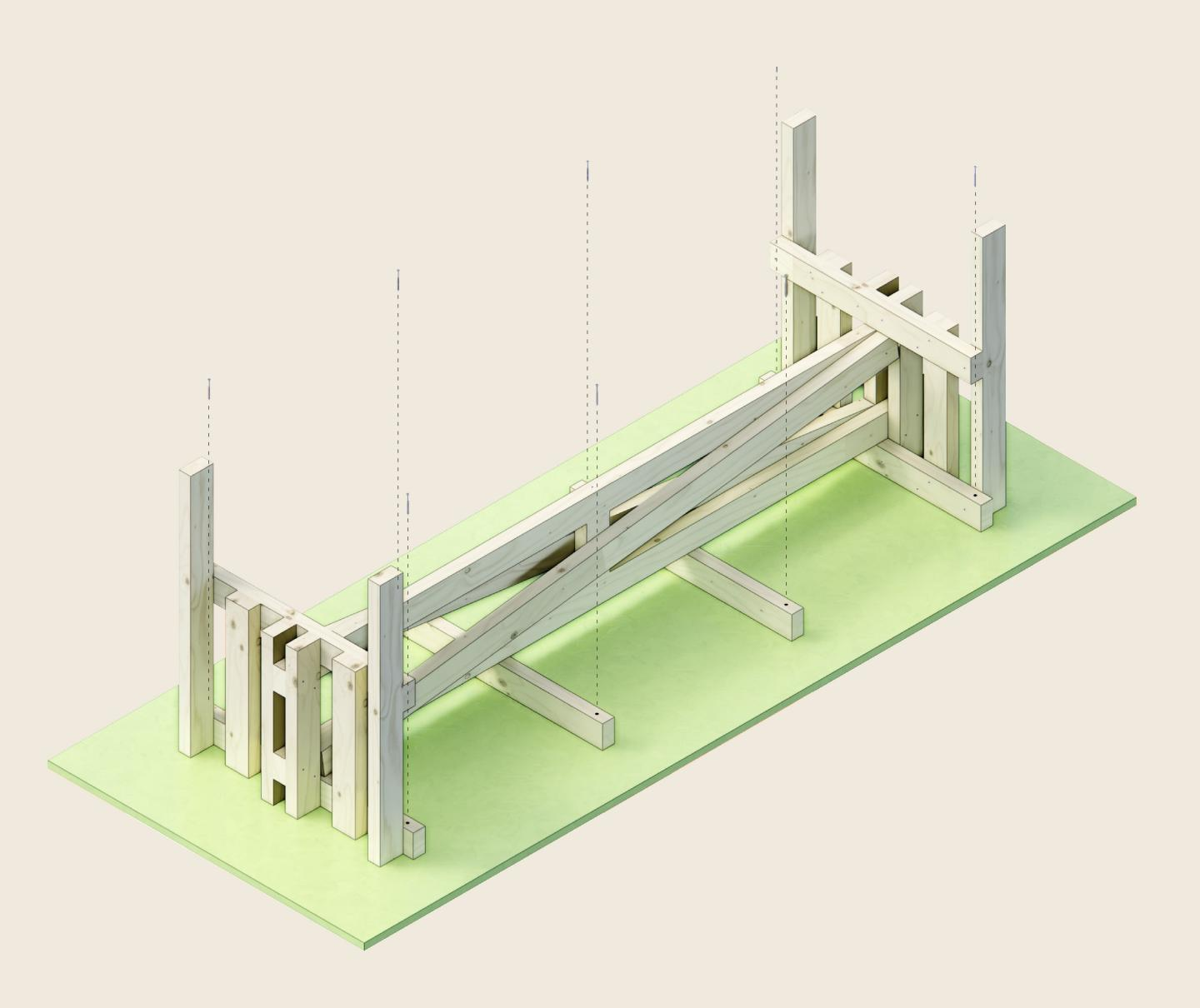
Make sure the middle battens are parallel to the rest of the frame before fastening with 90mm screws.
